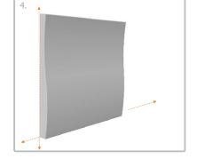
5. Install other panels so that they align with the first panel and horizontal/vertical lines. For each panel, press at all corners for 5 to 10 seconds.
