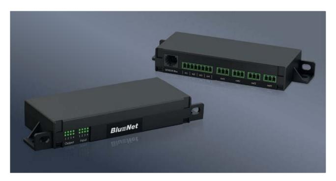
The GPIO Module (GPIO: general purpose input/output) allows you to expand BlueNet BN3000 – BN7500 PDUs by adding external sensors and/or actuators. Floating contacts provided on-site can then be queried and evaluated, and signalling can be performed via internal relay contacts, for example. Furthermore, it enables a physical connection to be established with the building control system for issuing alarms in response to set threshold values, such as when the residual current is exceeded.
