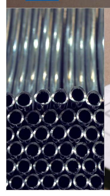
The main materials used in our products are steel, injected aluminium, upholstery and polypropylene. We specialise in all processes related to tubes, such as cutting, grinding, welding, punching machines and bending machines. The paint work is also one of our main processes, always using epoxy paint (2 coats + enamel).
