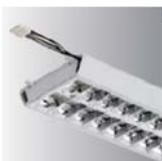
Miva Line is supplied with 7-pole through wiring with fast connectors which allows fast and simple line connection. This also allows many different switching possibilities or connection to dimmable systems and integration of emergency modules.
