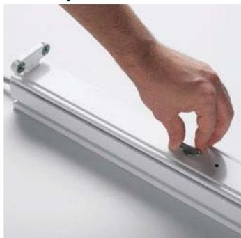
All luminaire inserts modules are easy to install thanks to simple 'twist & lock' operation. Just 90° turn is needed to lock the gear tray to the supporting rail.
