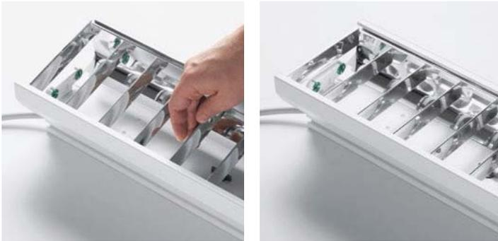
After external reflector alignment we can insert the parabolic louvre. Louvre mounting demand soft inclination during insertion. Louvre lapel keeps louvre safe in position.
