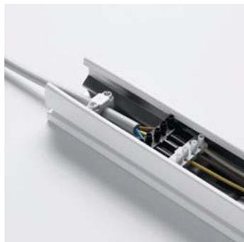
Cable entry into starting rail can be realized from upper side or through the end cap. Enclosed 5-pole quick connector enables fast and easy rail connection
